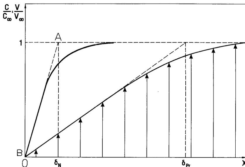
FIG. 3. Normalized concentration and velocity profile in a laminar flow at the sensor surface.
