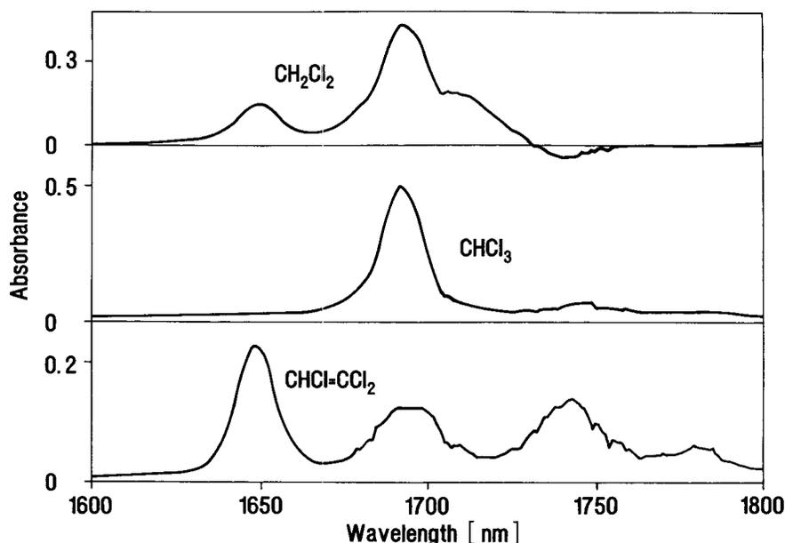
FIG. 4. Evanescent field absorption spectra of aqueous solutions of  $\text{CH}_2\text{Cl}_2$  ( $0.188 \text{ mol L}^{-1}$ ),  $\text{CHCl}_3$  ( $3.95 \cdot 10^{-2} \text{ mol L}^{-1}$ ), and  $\text{CHCl}=\text{CCl}_2$  ( $4.07 \cdot 10^{-3} \text{ mol L}^{-1}$ ); 6.43-m length/500- $\mu\text{m}$ -o.d. cladding/400- $\mu\text{m}$ -o.d. core fiber sensor.
