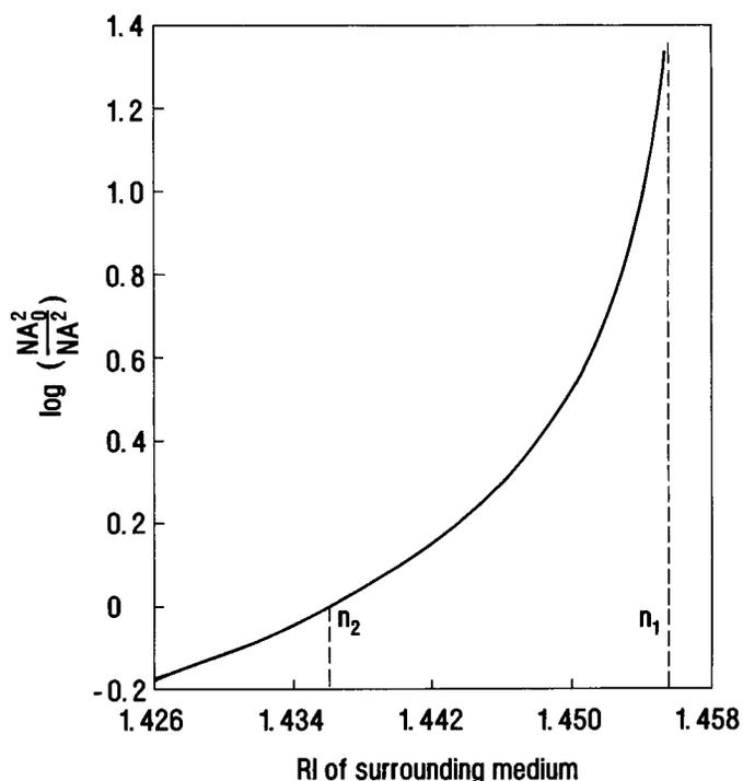
FIG. 2. Calculated contribution of the refraction term of Eq. 7 to the sensor response.
