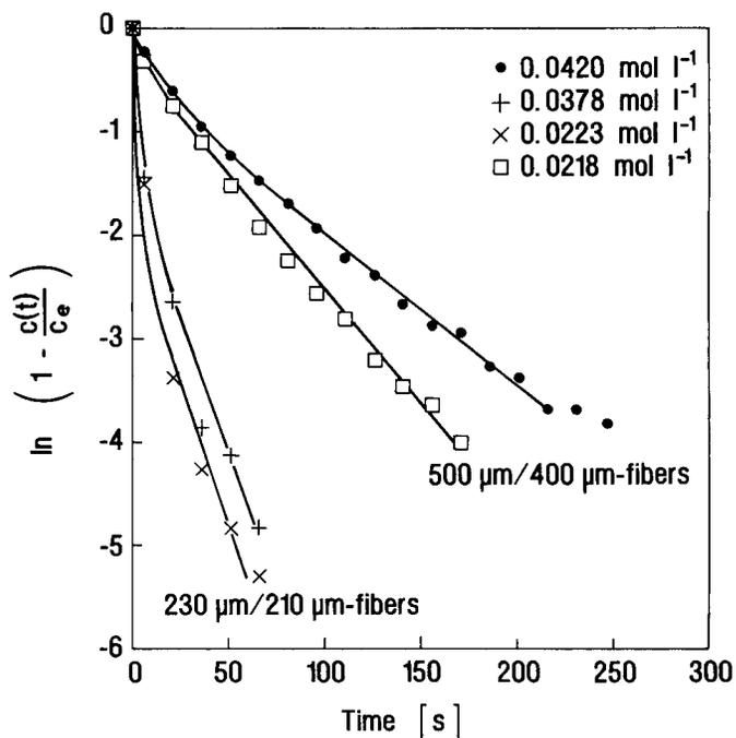
FIG. 11.  $\ln(1 - c(t)/c_e)$  values of a 210- $\mu\text{m}$  core and 400- $\mu\text{m}$  core fiber sensor for several  $\text{CHCl}_3$  concentrations.
