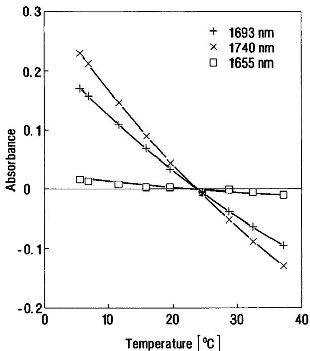
FIG. 6. Temperature dependence of the sensor signal at wavelengths of 1655, 1693, and 1740 nm; 6.43-m length/500- $\mu\text{m}$  cladding/400- $\mu\text{m}$  core fiber sensor in pure deionized water.
