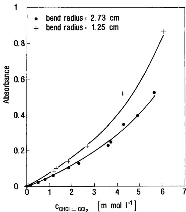
FIG. 8. Absorbance signal of a 6.43-m length/500- $\mu\text{m}$  cladding/400- $\mu\text{m}$  core fiber sensor for several bend radii.
