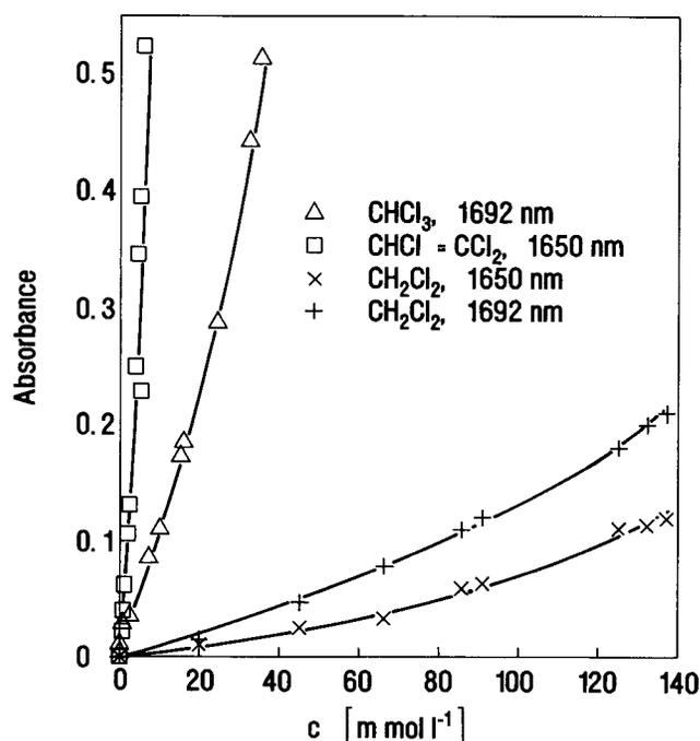
FIG. 5. Evanescent field absorbance signal of a 6.43-m length/230- $\mu\text{m}$  cladding/210- $\mu\text{m}$  core fiber sensor vs. molar analyte concentration in the aqueous phase for  $\text{CH}_2\text{Cl}_2$ ,  $\text{CHCl}_3$ , and  $\text{CHCl}=\text{CCl}_2$  at wavelengths of 1650 nm and 1692 nm.
