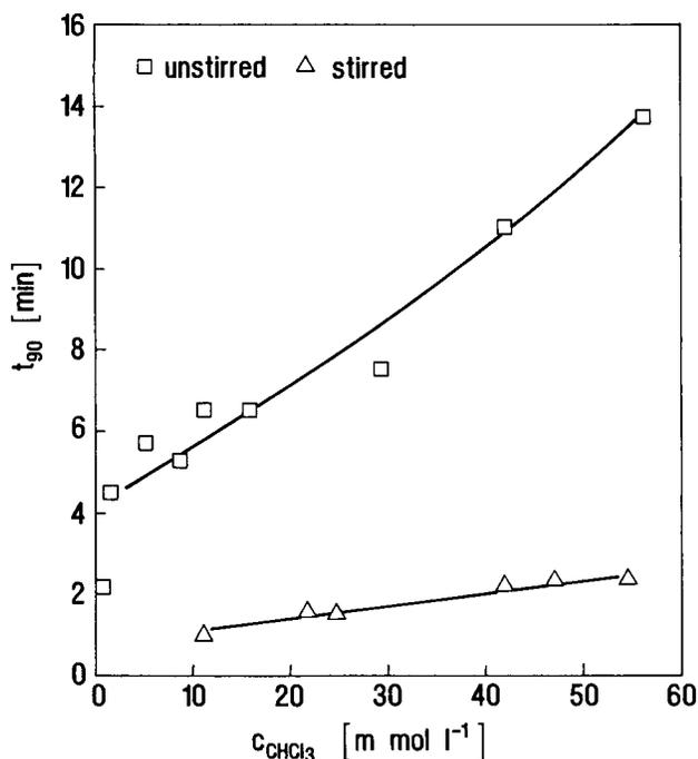
FIG. 10.  $t_{90}$  values of a 6.43-m length/500- $\mu\text{m}$  cladding/400- $\mu\text{m}$  core fiber sensor vs. molar  $\text{CHCl}_3$  concentration for stirred and unstirred solutions.
