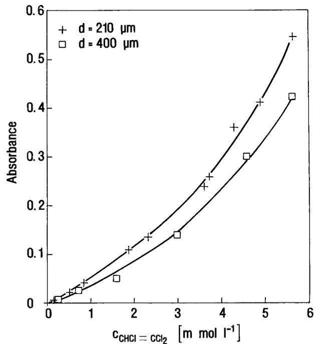
FIG. 9. Absorbance signal of a 6.43-m length sensor for several fiber core diameters.
