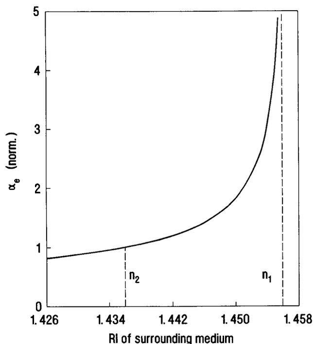
FIG. 1. Calculated normalized effective absorptivity  $\alpha_e$  vs. refractive index of the surrounding medium (cladding plus analyte).
