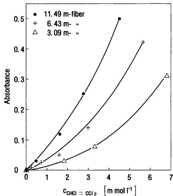
FIG. 7. Absorbance signal of a 500- $\mu\text{m}$  cladding/400- $\mu\text{m}$  core fiber sensor vs. molar  $\text{CHCl}=\text{CCl}_2$  concentration for several fiber lengths.
